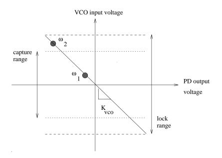
Figure 2: Phase-space diagram of lock range, capture range, and circuit state. State variables are the voltages labeled  $V_{PD}$  and  $V_{VCO}$  in the previous figure.
