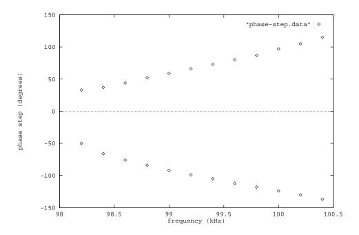
Figure 8: The maximum phase step that a locked loop can withstand, as a function of frequency. The edge of the lock range is 98.1kHz and the edge of the capture range is 100.8kHz
