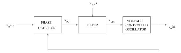
Figure 1: Phase-locked loop block diagram
